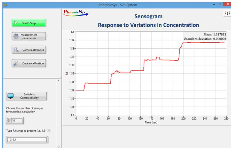
Translation from RI units to concentration units can be done easily using a simple formulae or a numerical table. Because of the continuous reference, the thermal fluctuations and drifts are compensated.
